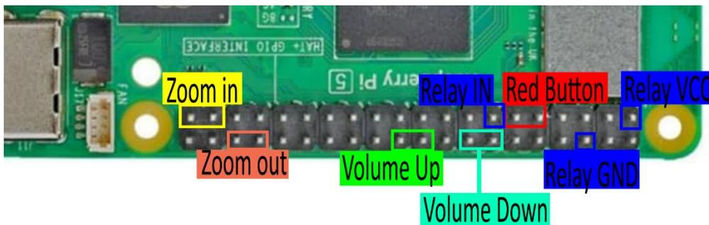
**Step 2.** Connect the three leads from the GPIO pins to the VCC/IN/GND side of the relay.
