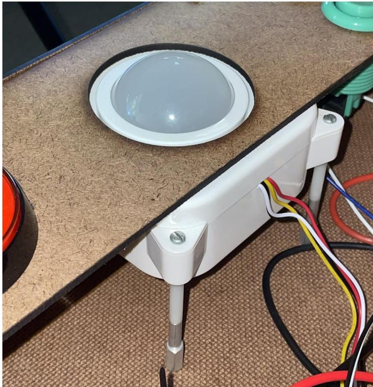
**Step 7.** Locate your 5 buttons (1 large, 2 small green, 2 small white). For each button, unscrew the fastener and insert the button through one of the holes in the last wood panel yet to be mounted. It doesn't matter which side is which color, though the buttons on the same side should be the same color. Install the large button in the smaller of the two center holes. Secure the buttons onto the wood plate by putting the fasteners back on.
