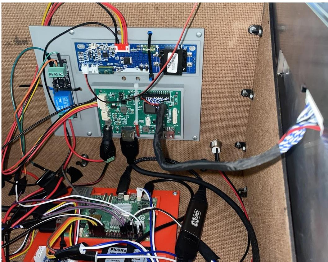
**Step 4.** Before mounting the monitor, try plugging in the device using the power adapter and test if it works. Note that the braided monitor cable is very short. You may want to provide additional security for it, or buy a longer one. As it is now, it's a good idea to physically hold it in place as you align the monitor.
