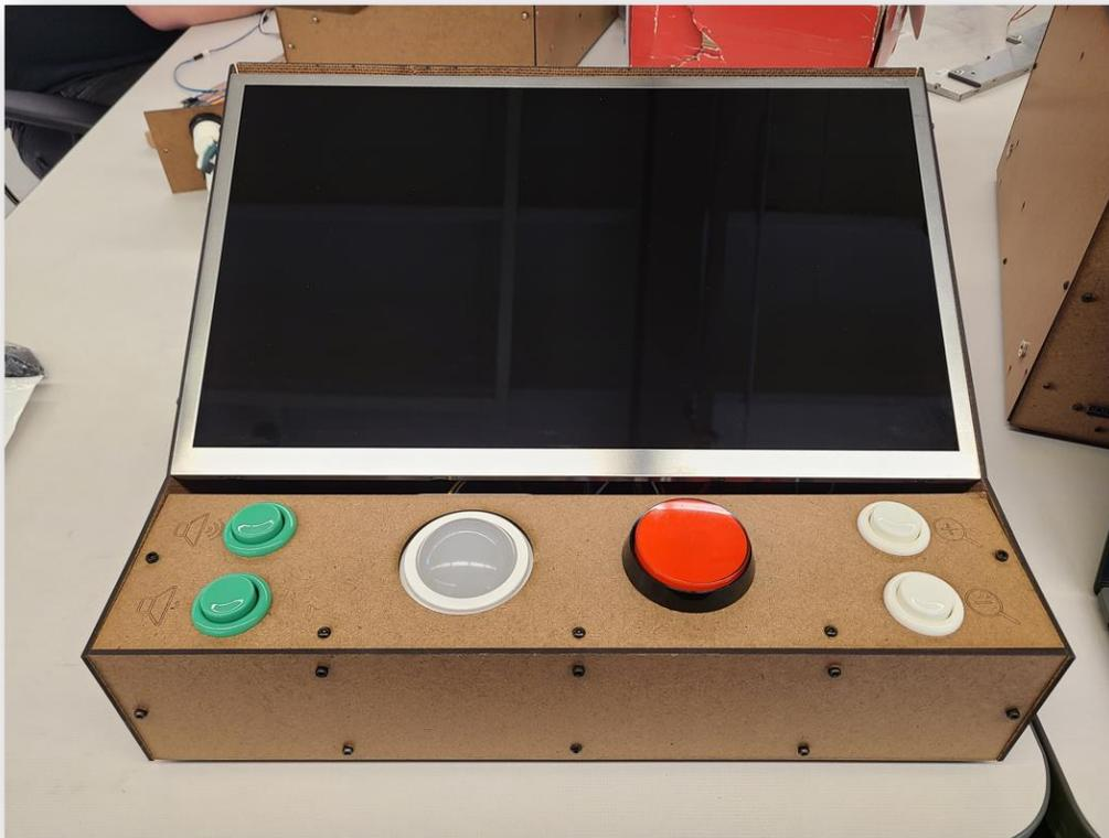
Figure 5: Side view of the current wooden testing chassis, with mounted components.
