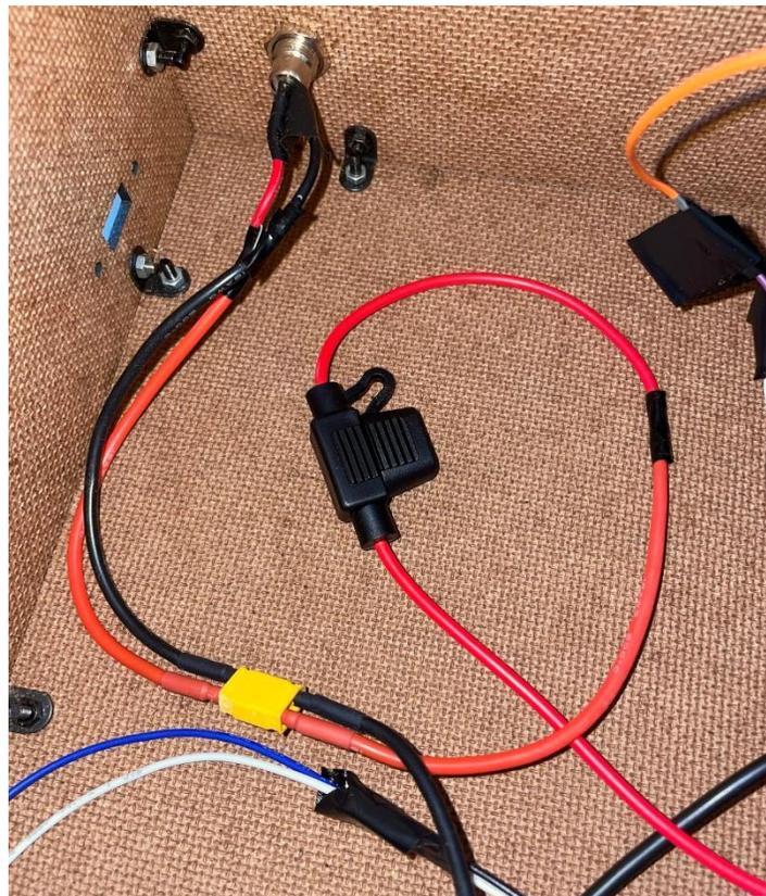
**Step 5.** Take its ends and split the power and grounds. That is to say, the one XT30 red cable needs to connect to two more red cables, and black needs to do the same. For both red and black, one split cable should be extra 18awg wire, and the other should be the positive end of the buck down converter. Solder each split.
