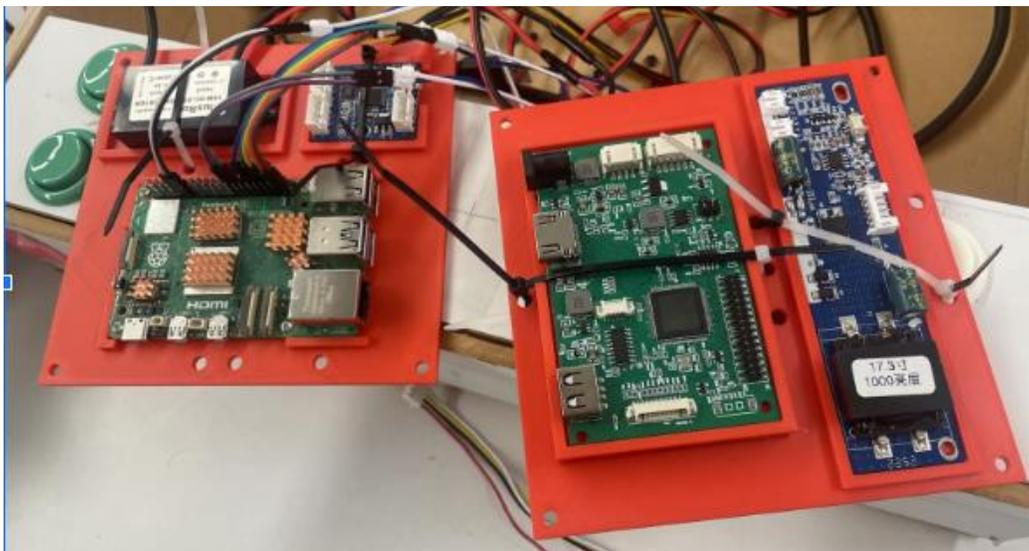
**Step 9.** Mount the 3D printed bracket to the back plate of the chassis. You can use any kind of screws/spacers/washers that fit, as long as the bracket is sitting a few millimeters above the chassis.
